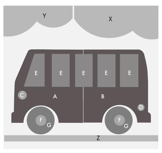
1. Cut sections A, B, E, X and Y from MDF or wood using the patterns on the following pages, noting the wood thickness needed for each piece before cutting. Combine A and B pattern pieces together before cutting.
